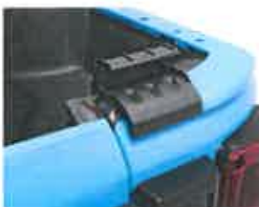
Use of tailgate bar and clips allows hassle-free opening of tailgate.
